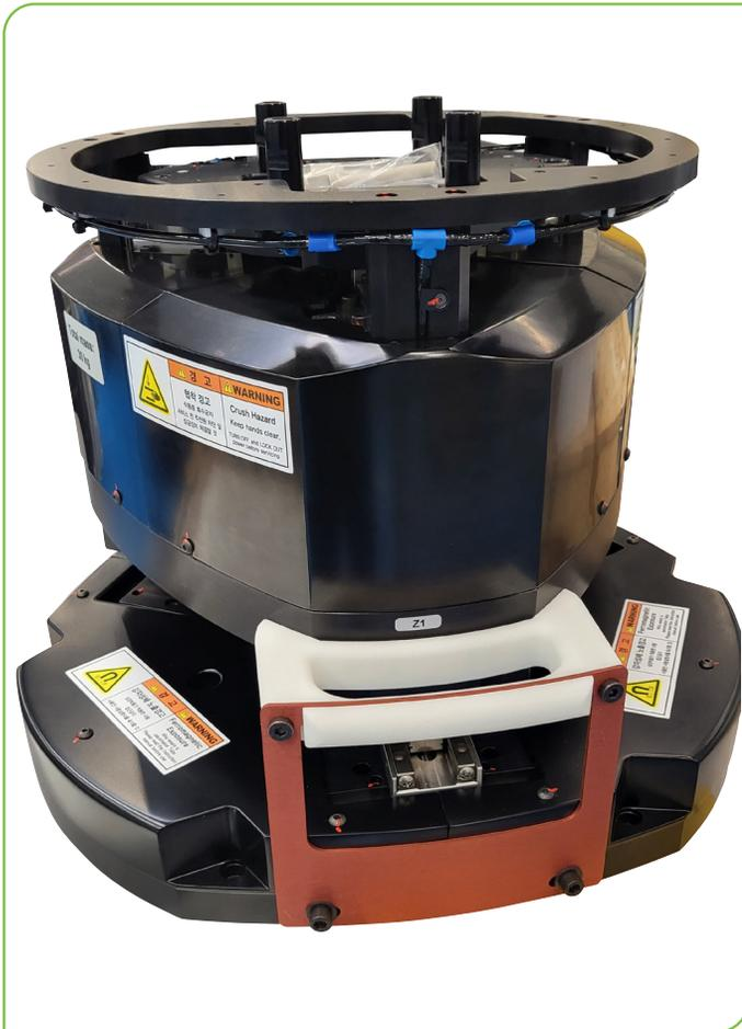
Parallel Robot for W2W Hybrid Bonding
